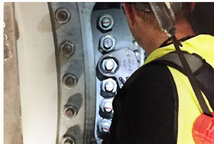
ITH Hydraulic Torque Wrenches Different designs up to 40,000 Nm (29,500 ft*lb)
