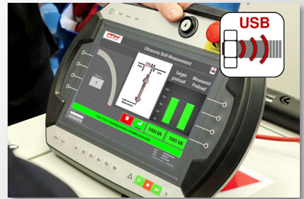
Ultrasonic Bolt Measurement System (USB) Digital measurements of the applied preload forces.
