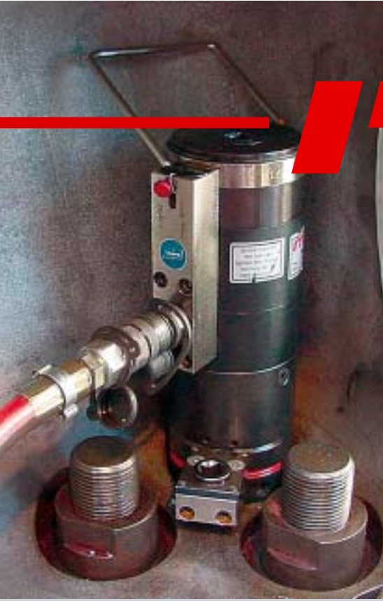
Loosening of CDC-bolts at GE turbine 7 FA + threads 2,0" - 8 UN with Multistage Bolt Tensioning Cylinder (BTC) MS - 200
